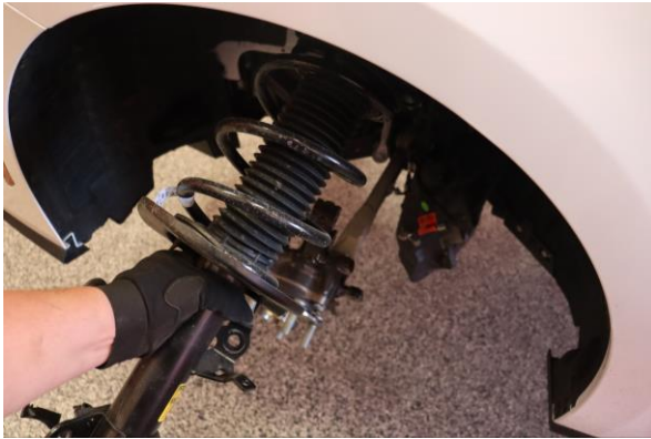
Step 13. Remove the shock assembly from the vehicle.
