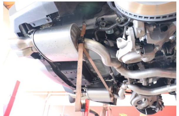
Step 12. Use a strap to support the exhaust.
