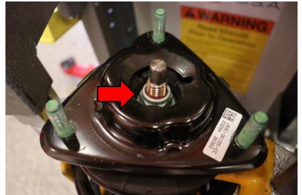
Step 16. Use a 21mm to remove the top hat mounting nut. Do not use an impact tool for this step, excessive rotation of the shock shaft during removal can damage the shock internal components. Hold shock shaft in place during nut removal to prevent damage.
