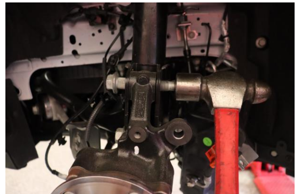
Step 10. Use a hammer to remove both lower shock mounting bolts.
