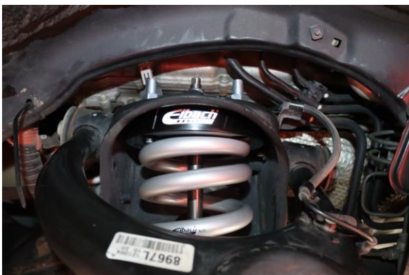
17. Install three upper shock mount nuts. Tighten to manufacturer specification.
