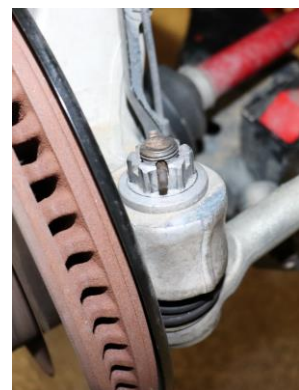
22. Install outer tie rod and upper ball joint cotter pins.
