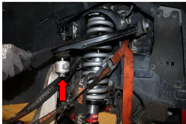
20. Use a pry bar to lower the upper control arm into the steering knuckle. Install the upper ball joint nut. Tighten to manufacturer specification.
