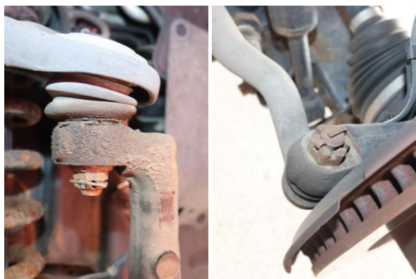
3. Remove cotter pins from upper ball joint and outer tie rod.
