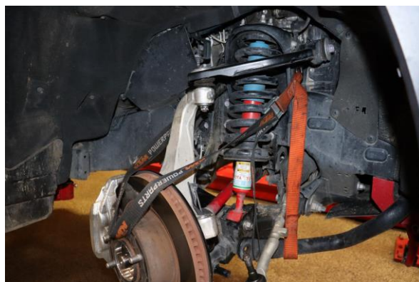
4. Use a strap to prevent damage to the axle when releasing upper ball joint.
