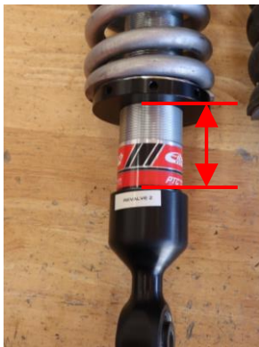
15. Verify pre-load before installing the PRO-TRUCK coilover by measuring from the bottom of the lower spring perch to the top of the lower shock mount. The default setting of 57mm should provide 1" of lift.
