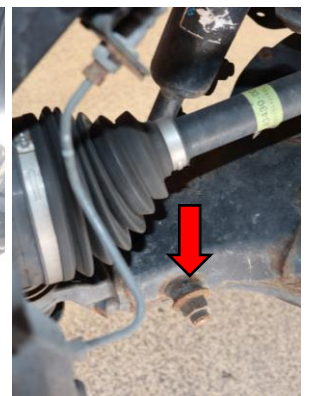
18. Install lower shock mount nut and bolt. Tighten to manufacturer specification.
