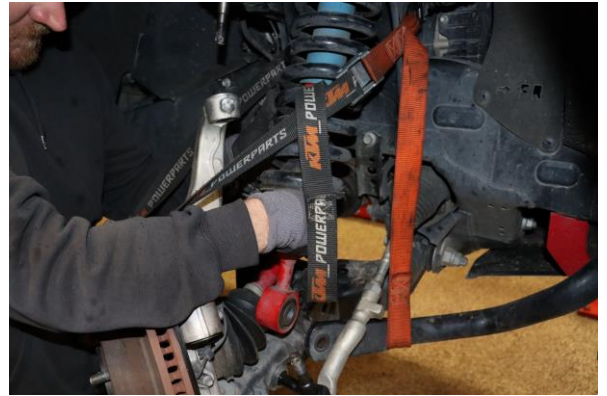
14. Push down on the lower control arm to release the lower shock bushing. Remove the shock assembly from the vehicle.
