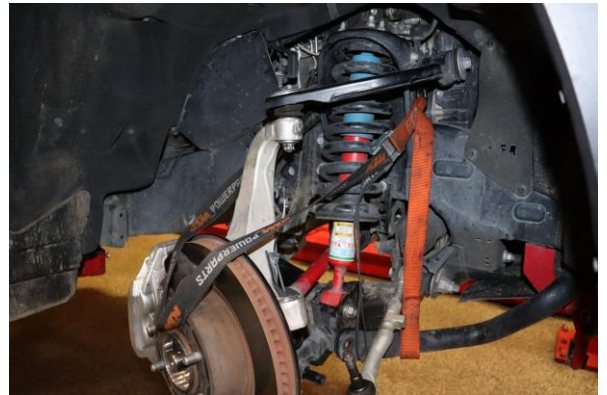
4. Use a strap to prevent damage to the axle when releasing upper ball joint.
