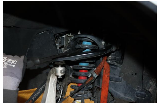
10. Use a pry bar to pull down on the upper control arm. Remove the upper ball joint nut and allow the steering knuckle to rest against the strap installed in step 2. Slowly allow the control arm and upper ball joint to lift from the steering knuckle.
