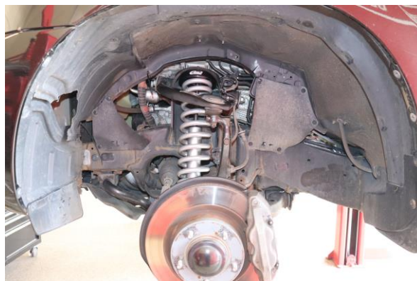
24. Remove the strap install in step 2. Install the wheel and tire. Tighten lug nuts to manufacturer specification.
