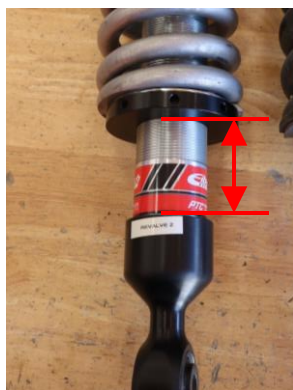
15. Verify pre-load before installing the PRO-TRUCK coilover by measuring from the bottom of the lower spring perch to the top of the lower shock mount. The default setting of 57mm should provide 1" of lift. This setting will provide a level lift with the OE rear spring. Adjustment will need to be made to achieve a level ride with Eibach rear spring.
