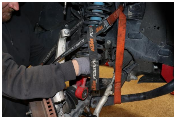
14. Push down on the lower control arm to release the lower shock bushing. Remove the shock assembly from the vehicle.
