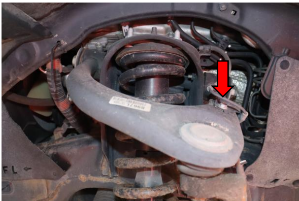
5. Remove bolt securing the wheel speed sensor wire harness to the upper control arm.
