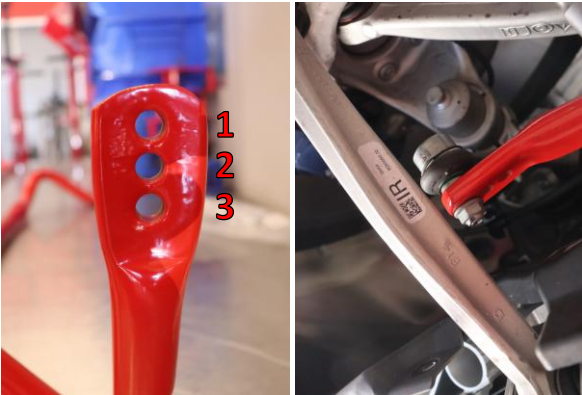
Step 15. Install the sway bar end link by selecting a setting. Setting one is the softest setting and setting 3 is the stiffest. Use a 16mm and T30 to tighten the sway bar end link to manufacturer specification.
