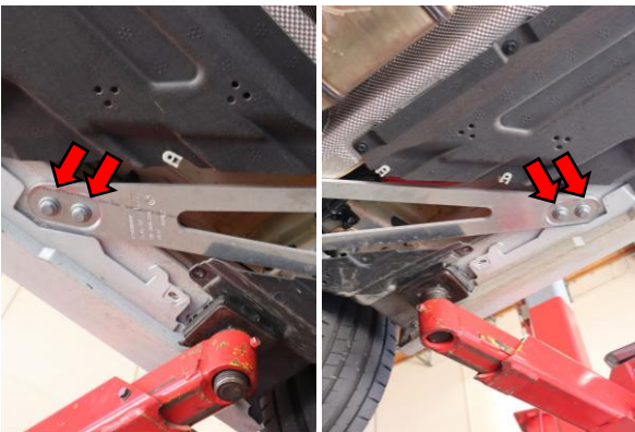
Step 17. Install the remaining bolts on the front aluminum belly pan. Tighten to manufacturer specification using 13mm.
