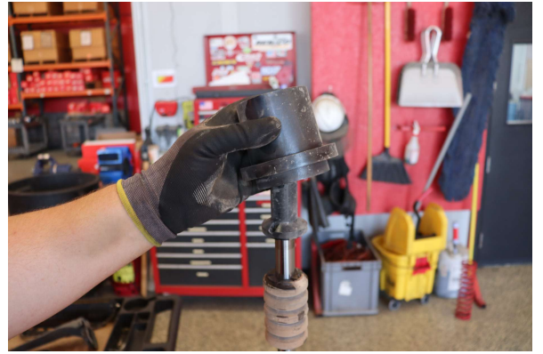
Step 8. Remove OE spring slider.
