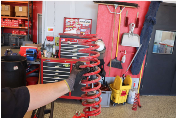
Step 7. Remove OE main spring.
