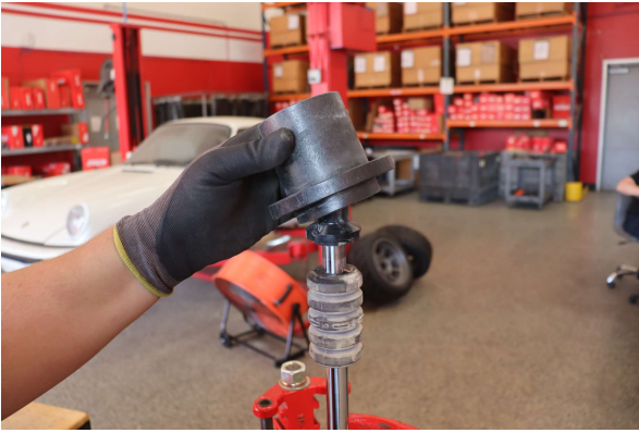
Step 13. Reinstall OE spring slider.
