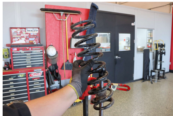
Step 8. Remove OE front main spring.
