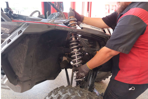
Step 17. Install shock in vehicle through the opening in the hood.
