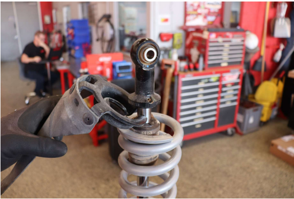
Step 15. Install lower spring retainer. Decompress spring assembly making sure that lower spring retainer and main spring sit flush with lower shock mount.
