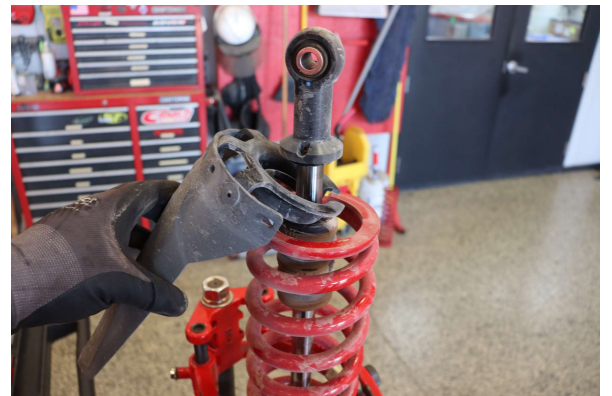
Step 6. Use a spring compressor to compress spring assembly. Remove lower spring retainer and decompress the spring.
