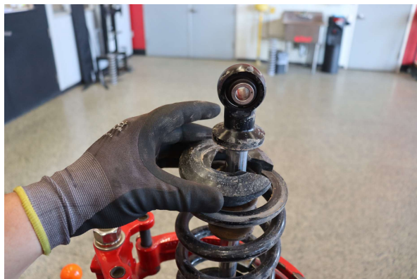
Step 7. Remove the lower spring retainer and decompress the spring.
