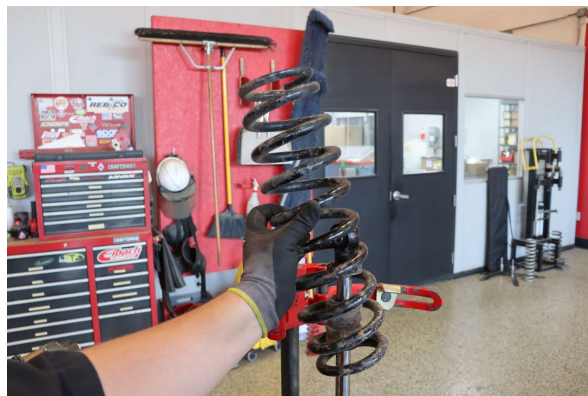
Step 8. Remove OE front main spring.
