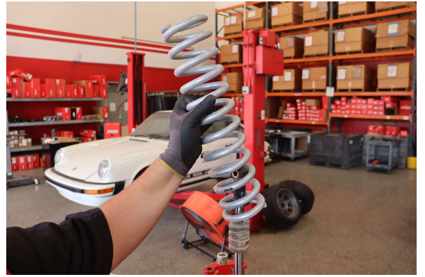
Step 14. Install Eibach main spring.
